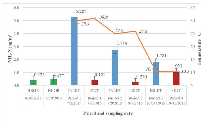
Ammonia concentration before and after treatment in the filter, the average temperature at the filter inlet and inside.
