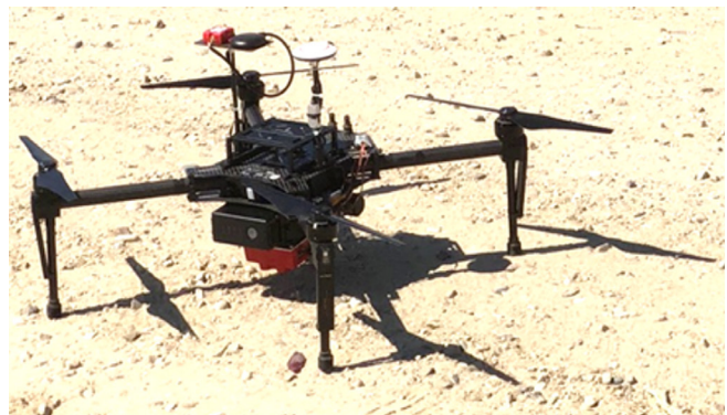
Figure 2. Matrice 100 UAV equipped with the RedEdge-M Camera.
