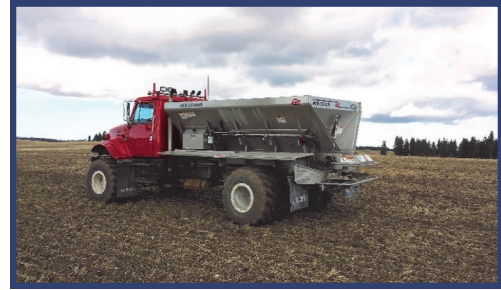
Figure 1. Lime was applied using a two-paddle distributor mounted on a "floater" truck.
